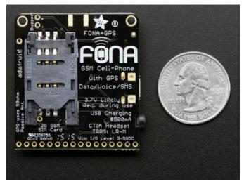
The SIM card holder is on the back. It holds a very-standard "Mini SIM"
