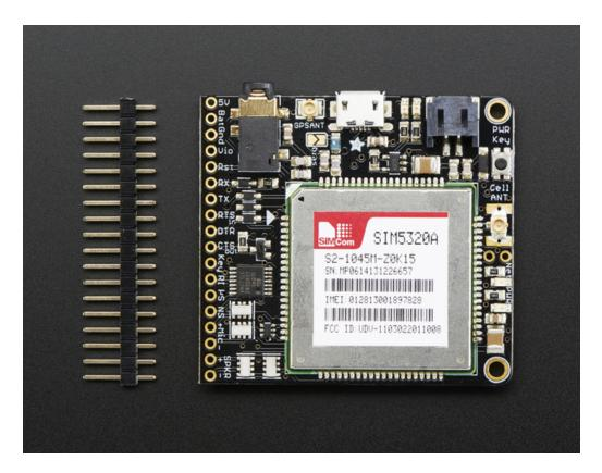
This module measure only 1.75"x1.6" but packs a surprising amount of technology into it's little frame. At the heart is a powerfull GSM cellular module (we use the latest SIM5320) with integrated GPS. This module can do just about everything
